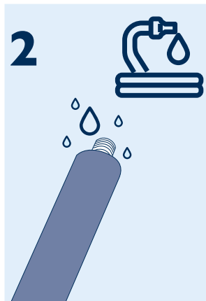
Wash with boiling soft water to remove salt deposited inside the coupling.
